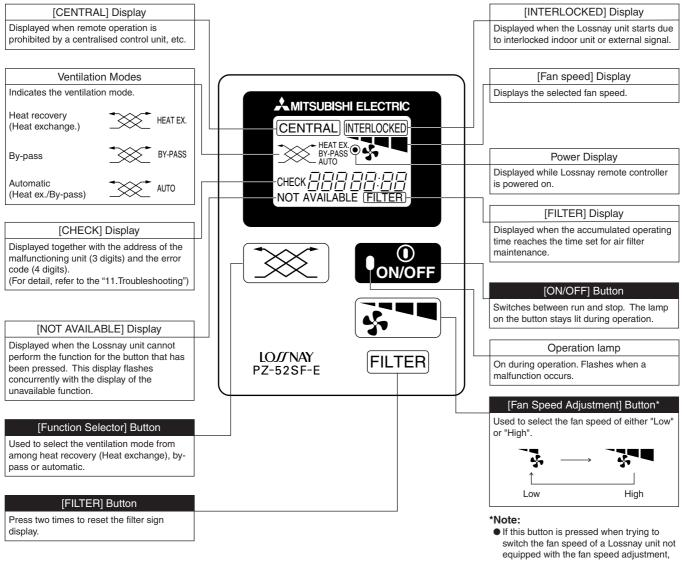
If this button is pressed when trying to switch the fan speed of a Lossnay unit noi equipped with the fan speed adjustment, the fan speed display and the "NOT AVAILABLE" display flash and the fan speed does not change.
