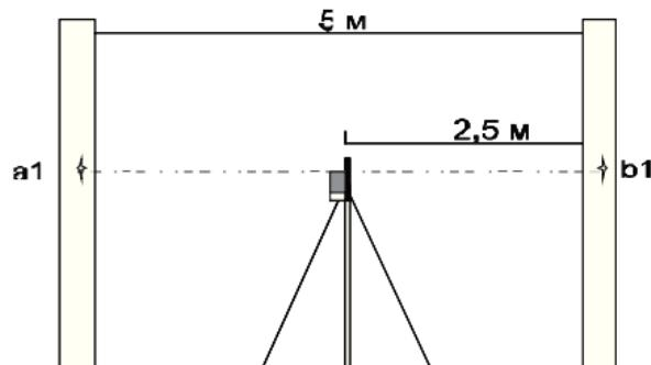
Set up the instrument 0,5-0,7m away from the wall and make, as described above, the same marks. If the difference  $\{a1-a2\}$  and  $\{b1-b2\}$  is less than the value of "accuracy" (see specifications), there is no need in calibration.
