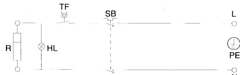
R-electric heating element; TF-thermostat;
