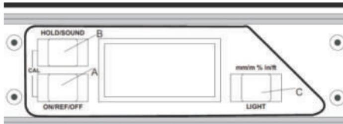
**3) Button C** converts angles to different units. Push once to change the display units from degrees ( $^{\circ}$ ) to mm/m, to percent slope (%), to pitch (in/ft). Hold button for 3 seconds to turn on light. Touch any key to illuminate the display while light function is on. Hold button again for 3 seconds to turn off light.
