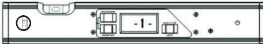
2. Rotate the level  $180^{\circ}$  in the same location and press A button, -2- will flash briefly. Do not move until the unit has completed the calibration and reset the display to the current level.
