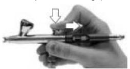
Press trigger to deliver air.
