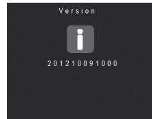
Press **M** to Menu mode. Choose **i** to indicate software version. Press trigger. Press **M** to exit.
