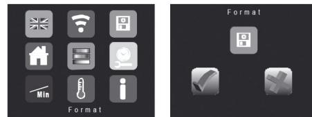
Press **M** to Menu mode. Press **◀** and **▶** or **▲** and **▼** to choose . Press trigger. Press **◀** or **▶** to choose to format. Press trigger to confirm. Press **M** to exit.
