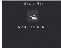
Press **M** to Menu mode. Press **◀** and **▶** or **▲** and **▼** to choose **Min**. Press trigger. Press **◀** or **▶** to adjust max. and min. temperature. Press trigger to confirm. Press **M** to exit.
