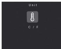
Press **M** to Menu mode. Press **◀** and **▶** or **▲** and **▼** to choose **Unit**. Press trigger. Press **◀** and **▶** or **▲** and **▼** to choose °C/F. Press trigger to confirm. Press **M** to exit.
