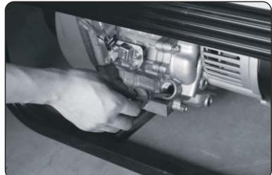
(b) Reinstall the drain plug and fill the engine with oil until it reaches the upper level on the oil filler cap.
