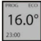
If the display shows PROG ECO, you can set the programming range in ECO mode. To change the temperature in ECO mode range, go to Temp. ECO menu (see “*Menu in PROG mode*” section).
