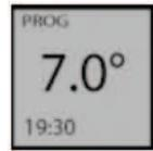
If the anti-freezing temperature (7°C) is set, then when switching to ECO mode programming range the display will show 6°C (*automatic decrease by 1°C*)
