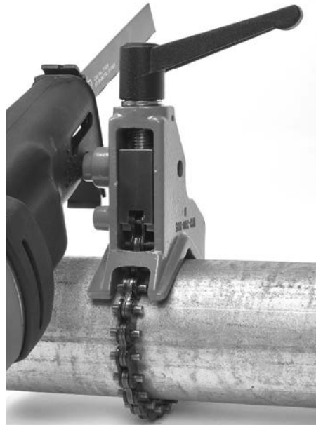
Figure 13 – Mounting Saw on Support Device
