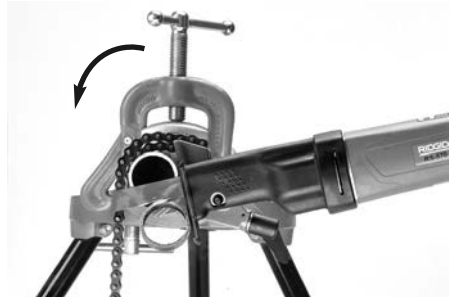
Figure 15C– Cutting the Pipe
