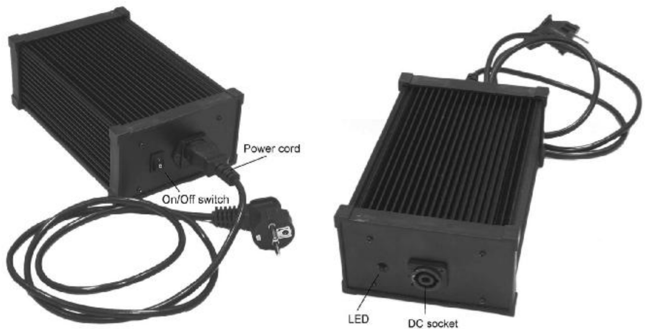
FIGURE 2. Power supply unit
